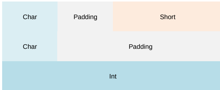
Figure 4-5: Structure with pragma pack with 4 byte alignment
