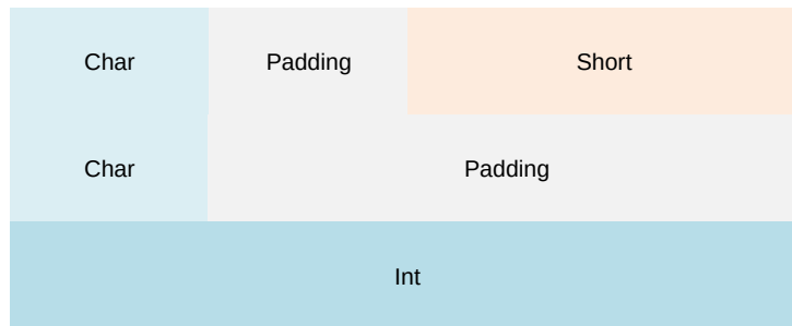
Figure 4-1: Structure without packing attribute or pragma
